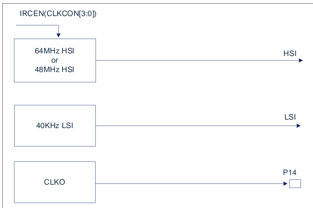
Figure3-1: Block diagram of the clock structure
